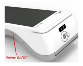
Sit the PAX A920 Pro terminal in the charging base, and power on the device by pressing the power button for 3 seconds. The power button is located on the right side of the terminal.
